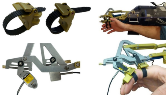
Fig. 1. Finger rehabilitation robot using motor and rigid transmission structure. 22
